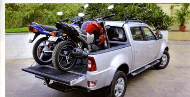
The Xenon's load bay is designed to carry 500kg. It is too shallow and too short because of the double cab's length.
