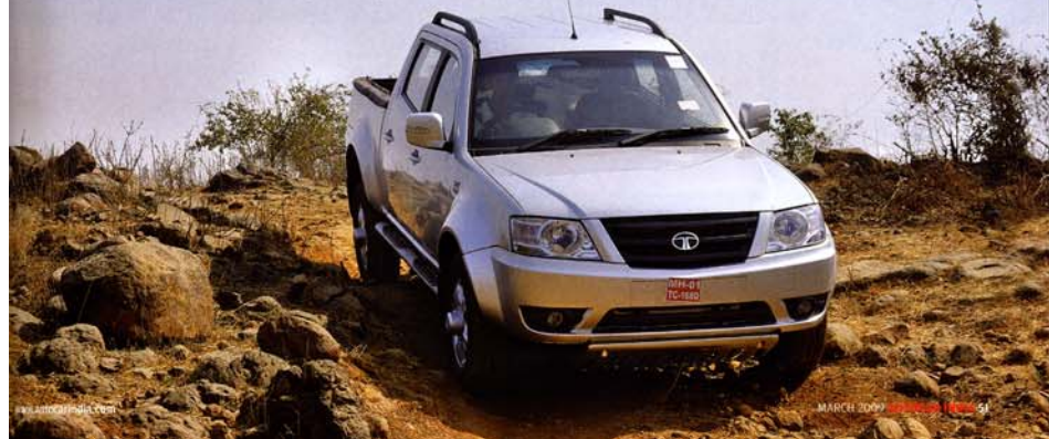
The Xenon's load bay is designed to carry 500kg. It is too shallow and too short because of the double cab's length.
